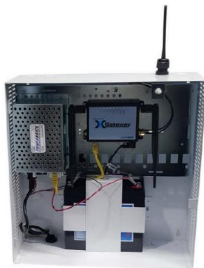
Figure 6: NAD Enclosure Example includes 4GSM Gateway and Power Server
